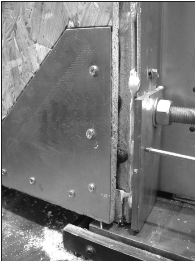
Figure 20. Tensile test on module with stiffening plate
